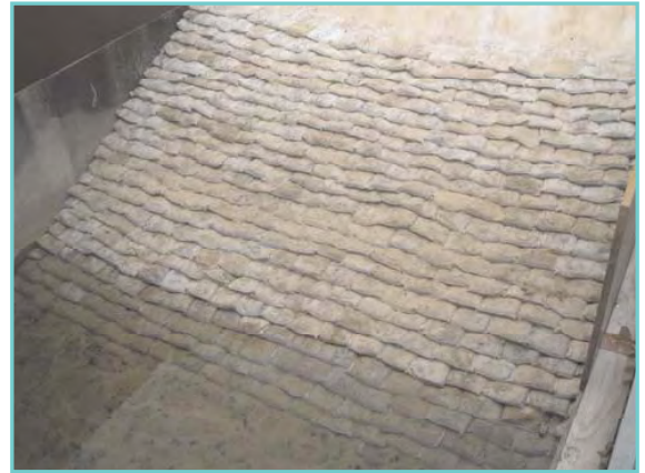
1:10 scale ELCOROCK ® containers in the flume ready for testing
